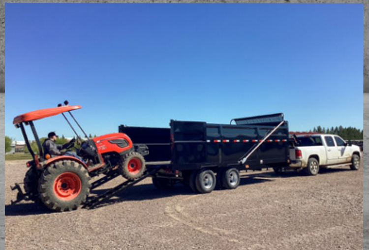
96" LONG 2 X 3 1/4" TUBING RAMPS
