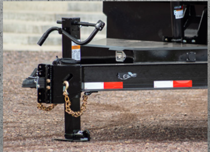
10K Drop Leg Jack W/ Adjustable Coupler
