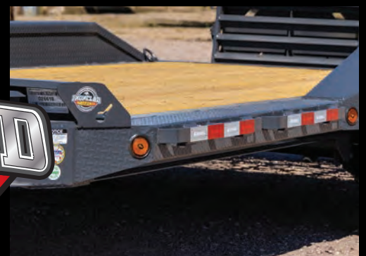
8" I-BEAM FRAME & RUB RAILS
