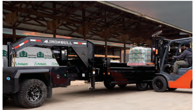
36" Deck Height, 18" Fold Down Sides
