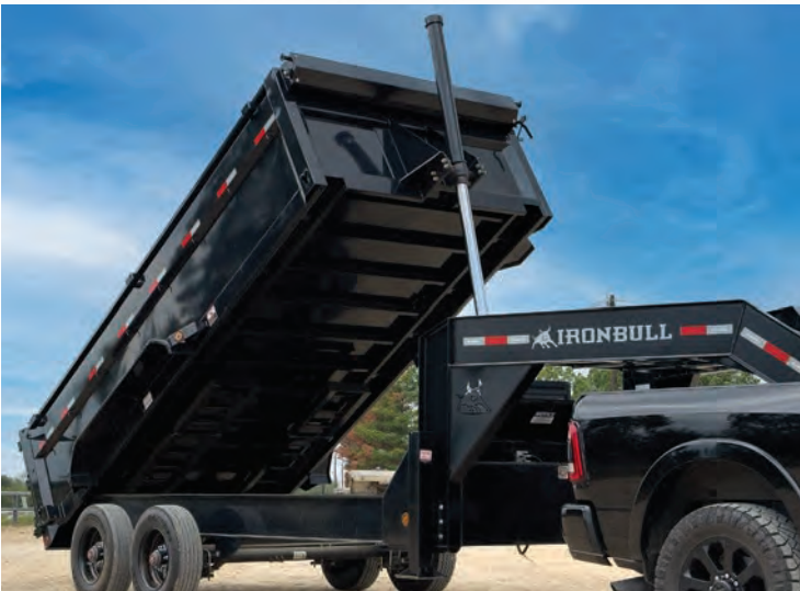
3 Stage Telescopic Cylinder (12 tons x 144")
