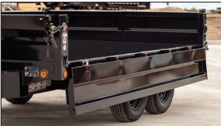
36" Deck Height, 18" Fold Down Sides
