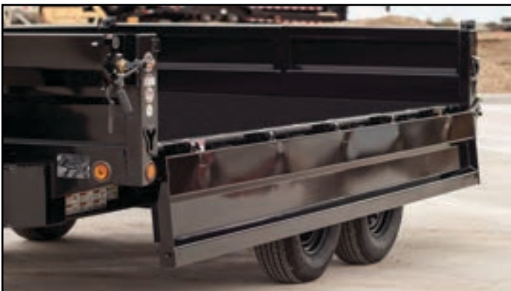
32" Deck Height, 18" Fold Down Sides
