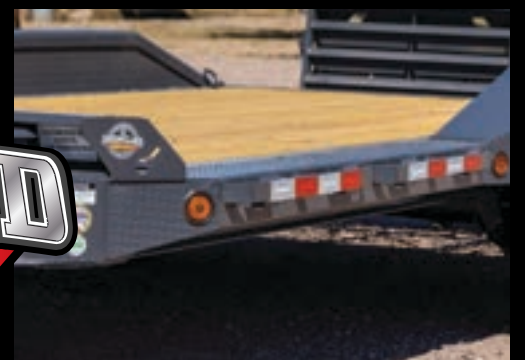
8" I-BEAM FRAME & RUB RAILS
