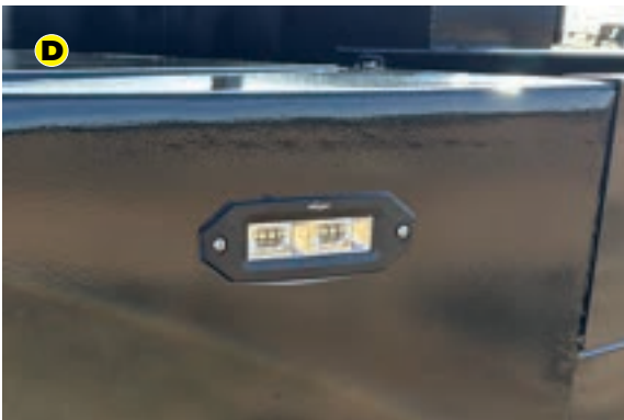
D FLUSH MOUNT REAR WORK LIGHTS, 3600 LUMENS
