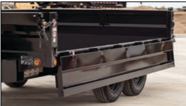
32" Deck Height, 18" Fold Down Sides
