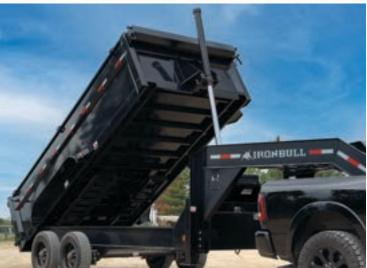
3 Stage Telescopic Cylinder (12 tons x 144")
