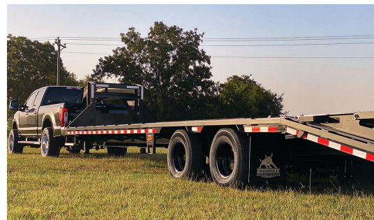
2 - 12k Electric Brake Axles
