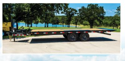
Our TDP14 Deckover features an 8" I-Beam tongue and frame. 14k GVWR and dual hydraulic cylinders with optional scissor. The TDP is built to deliver maximum performance and versitility.
