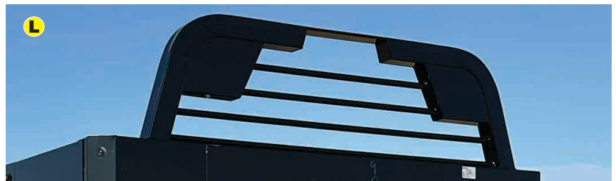
HEAD RACK NOTCHED FOR TRUCK 3RD BREAK LIGHT VISIBILITY
