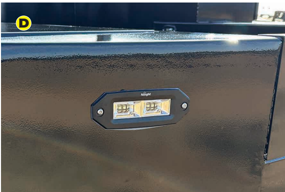
FLUSH MOUNT REAR WORK LIGHTS, 3600 LUMENS
