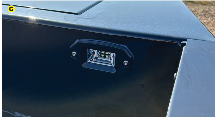
CARGO LIGHTS ON THE DECK/INNER CABINET
