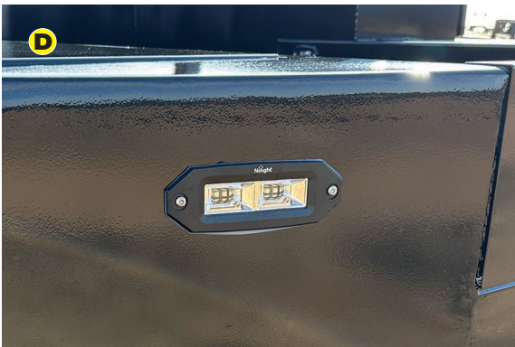
FLUSH MOUNT REAR WORK LIGHTS, 3600 LUMENS
