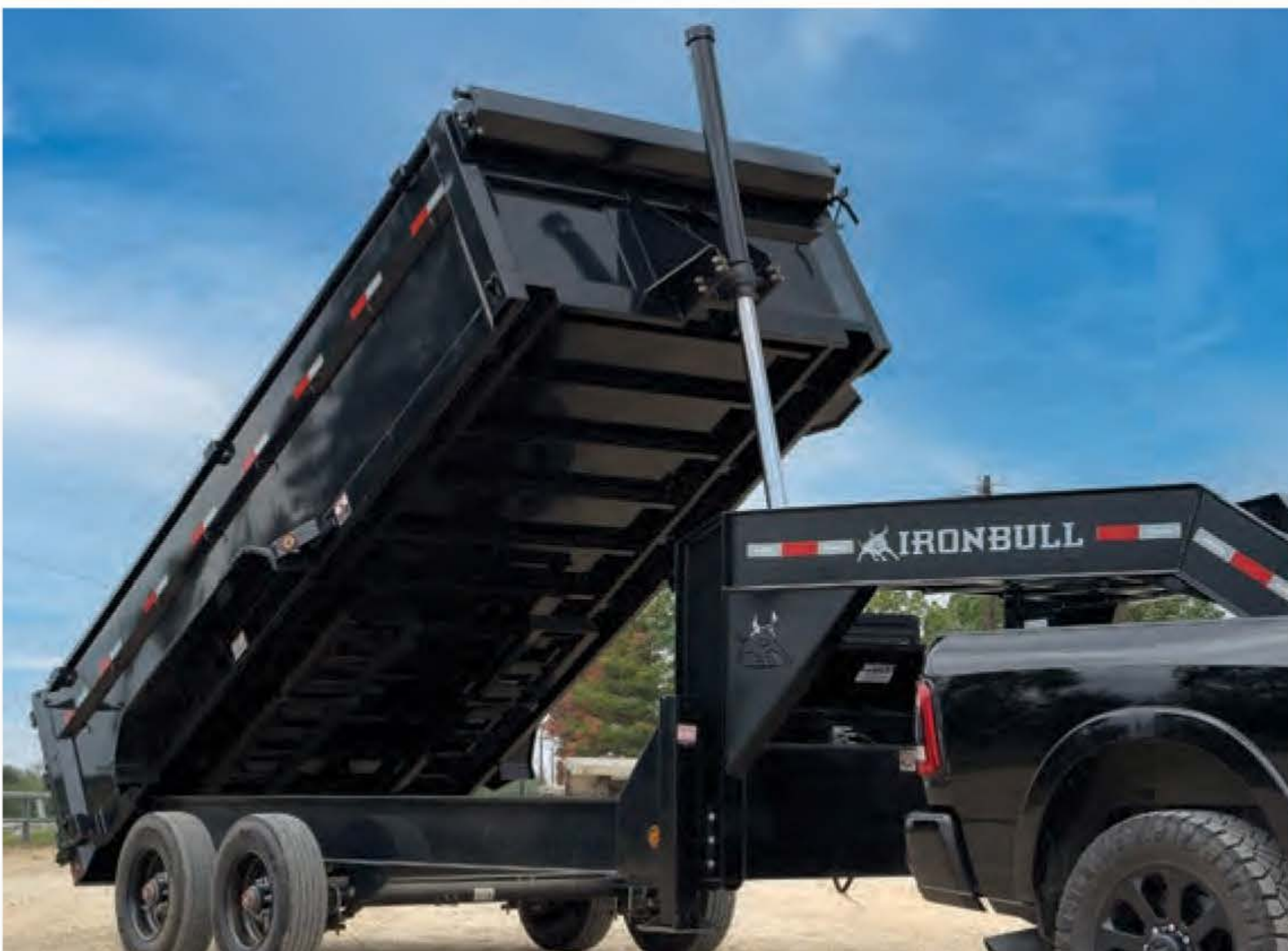
3 Stage Telescopic Cylinder (12 tons x 144")
